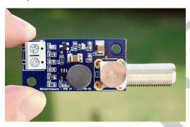
At PCB 20.1 and subsequent boards the free board space at PCB 20.x next to PCB 17.x is used as an experimental electrical antenna. This antenna is designed only for testing purposes. You can also bend these aerial and connect a long wire antenna at the two pin header. The external connection point is ground, the central connection point is the antenna. Note that any electrical antenna must be placed outside far away from from buildings and electrical interference sources.
