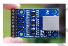
The antennas are connected to the pre-amplifier as follows from left to right if viewed from above if the terminal block is directed upwards. Any polarity between A1/A2, B1/B2, and C1/C2 does not matter.
